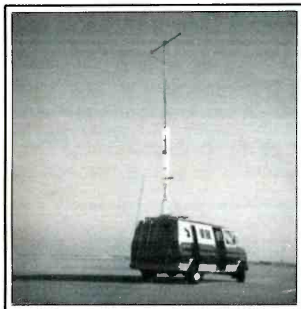
John (SSB-329B) went whole-hog with a 15-foot foldaway tower 45 feet in the air. This is topped with a V-Quad antenna.
