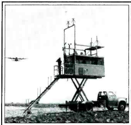
The ATC/4952/M is cleverly designed so that it can be a fully-functioning combat zone control tower within moments after arriving on the scene.
