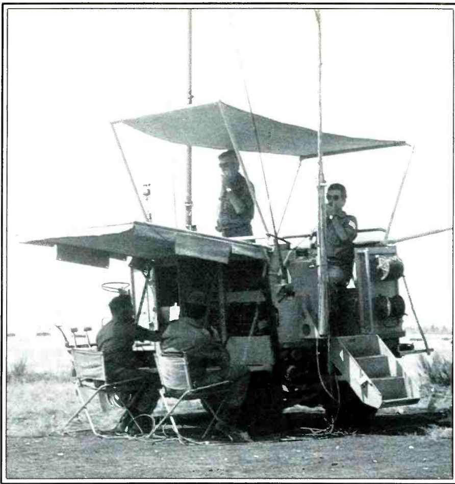
It's hard to believe that only a few moments before this picture was taken this was little more than a jeep. Now it's a complete mobile communications center and air traffic control tower. This unit is called the ATC/4950/AM.
